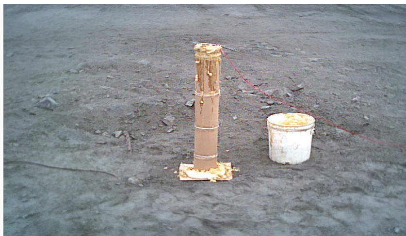
Figure 1. External appearance of experimental charge in a cardboard shell of 130 mm diameter
